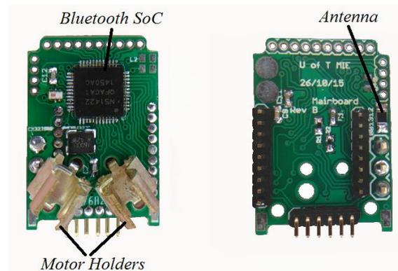
Figure 3. Mainboard module circuit board (back and front views).
