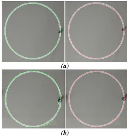
Figure 7. Circular path tests for (a) *mROBerTO* and (b) *Kilobot*.
