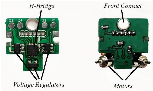
Figure 4. Locomotion module circuit board and motors.
