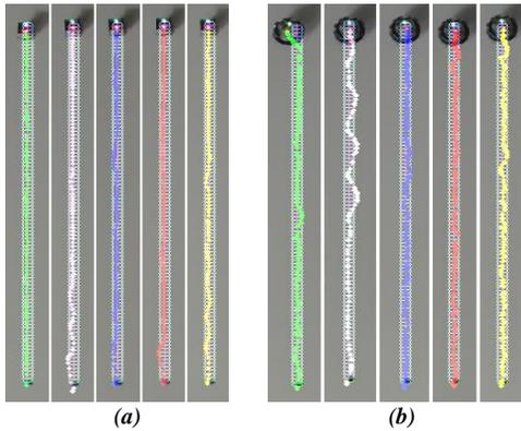
Figure 6. Straight-line tests for (a) *mROBerTO* and (b) *Kilobot*.
