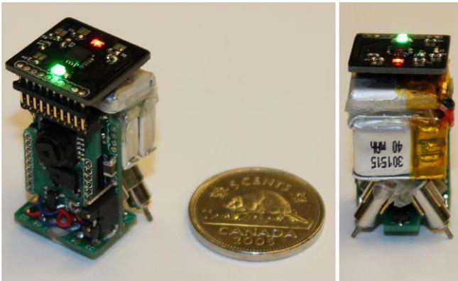
Figure 1. *mROBerTO* shown next to a Canadian nickel (diameter of 21.2 mm) for scale.
