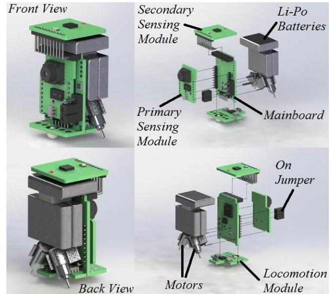
Figure 2. *mROBerTO*'s exploded-assembly view.
